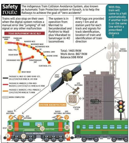
into them. One of its features is that by continuously refreshing the movement information of a train, it is able to send out triggers when a loco pilot jumps signal, called Signal Passed at Danger (SPAD).
